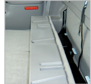
The DU-HA bolts to rear floor flaps to allow access to the jack when tilted forward.
