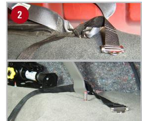
Photo shows two models of seat belt brackets, straps should loop through.
